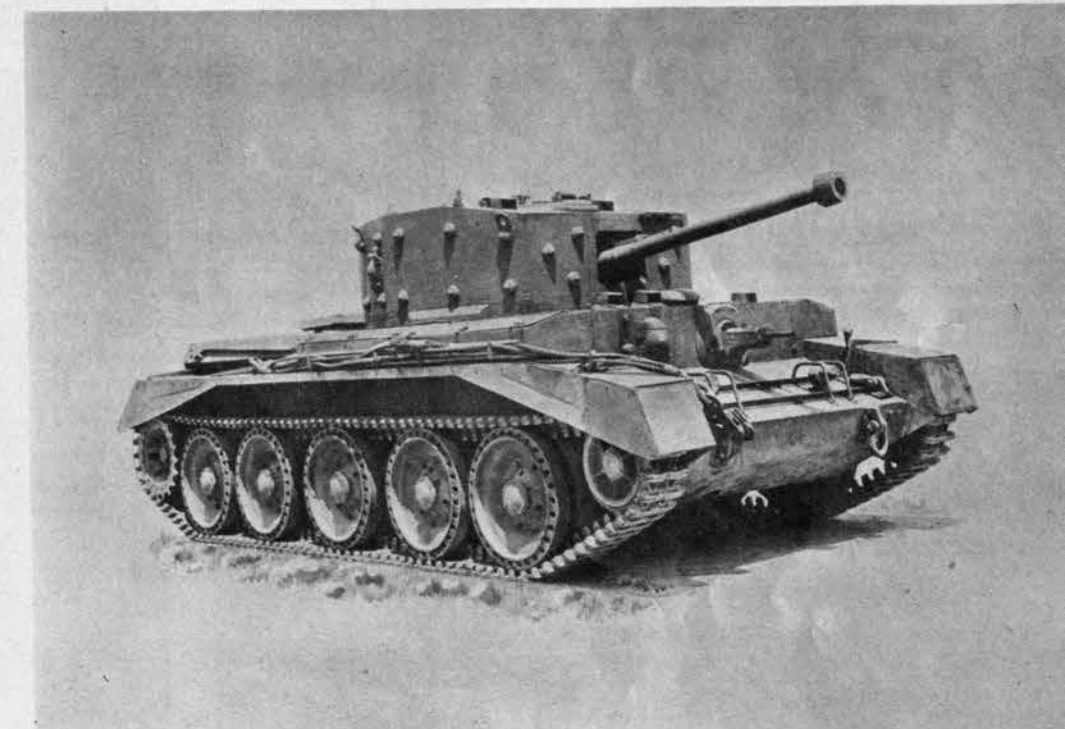
British Cromwell doesn't have T-34's wide track but has borrowed its five large wheels, high-set front idler and rear driving sprocket. Churchill (below) is unusual in having eleven small bogie wheels, very high rear sprocket and front idler, and long, overall tracks.
